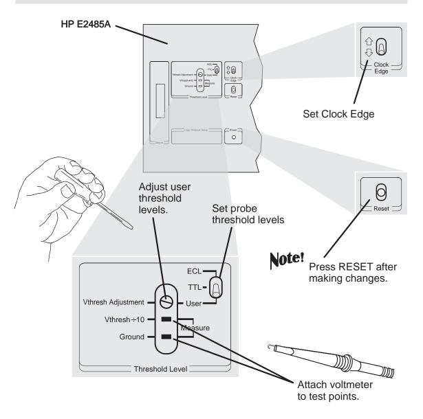
Vthresh is the threshold voltage of your target system. Data sent from the HP E2485A to the logic analyzer use TTL logic levels.
